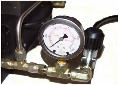
Step 6. Slowly open the fill lever (Figure 14) to allow pressure from the paintball cylinder to equalize the pressure in the fill line from the Megabooster to the paintball cylinder. At this stage note the pressure on the Megabooster gauge. DO NOT pay attention to the gauge on the paintball tank, the Megabooster gauge is much more accurate.
