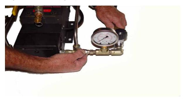
Step 3. Locate the output side (Figure 6) and install the compression fitting the same as with the inlet side, also torquing the compression nut to 20 ft/lbs. Correct placement of the outlet side can be seen in Figure 6. Once this is accomplished, the holes for the U-bolts (provided) can be drilled and the U-bolts installed, as in figure 4. Again, ensure the flat plates are installed on the bottom of the U-bolts underneath the mounting surface before the nuts are installed.
