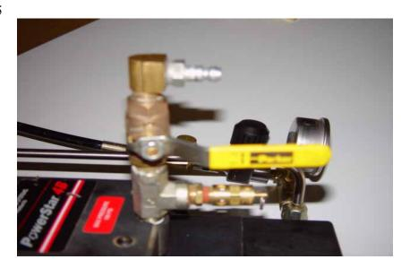
Step 7. Slowly open the drive air valve (Figure 15) allowing the Megabooster to begin operation. Pay careful attention to the Megabooster pressure gauge, as the gauge will climb very quickly if the paintball cylinder valve is not open. Slowly open the drive air valve, filling the cylinder. As the pressure approaches the rating of the cylinder, slowly begin to close the drive air valve, "throttling" the speed of the Megabooster as the pressure approaches the rating of the cylinder.
